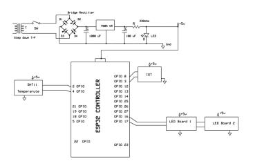
Fig 1; Block diagram
